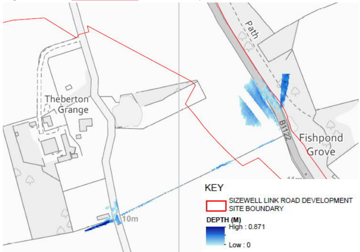
Plate 4.24-22: Maximum flood depth in the with scheme scenario for crossing 7 – 1 in 100-year event with 65% climate change (extract from Figure B7.9 in APPENDIX C: APPENDIX C )
